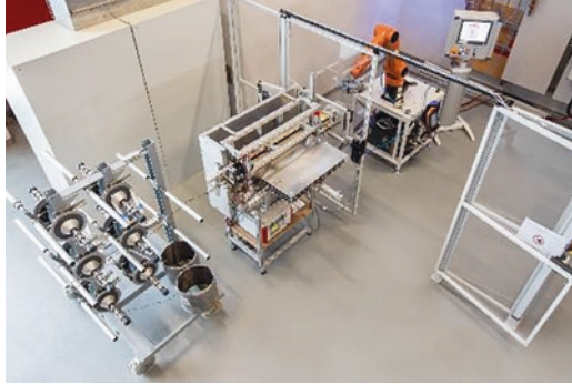
Fig. 2. 3D skeleton winding prototype line at Fraunhofer ICT
