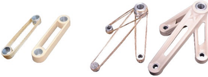
Fig. 4. Simple loop structure before/after overmolding with PPS (left), and 3D generic component before/after overmolding with PPS (right)
