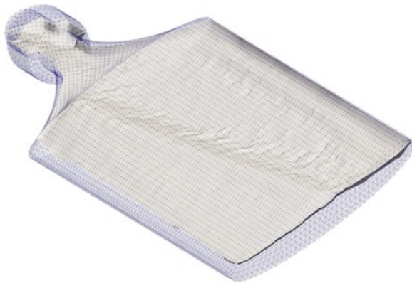
Fig. 6. Illustration of the resin flow during a time step of the rotational moulding simulation on the example of a rotor blade used for the construction of ventilation fans
