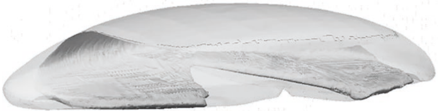
Fig. 5. Illustration of the resin flow during a time step of the rotational moulding simulation on the example of a white water kayak
