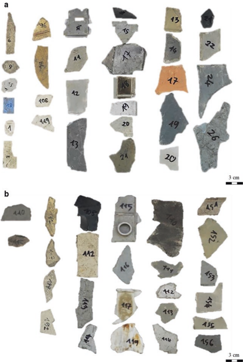
Fig. 1. Example of the reference plastic waste particles of shredded shells of cathode ray tubes (television apparatus), adopted to define the training (a) and the validation dataset (b).
