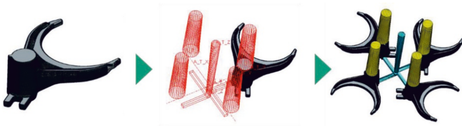
Fig. 2. Modified model for casting simulation (left: forging part, centre: the new injection system, right: cast model)
