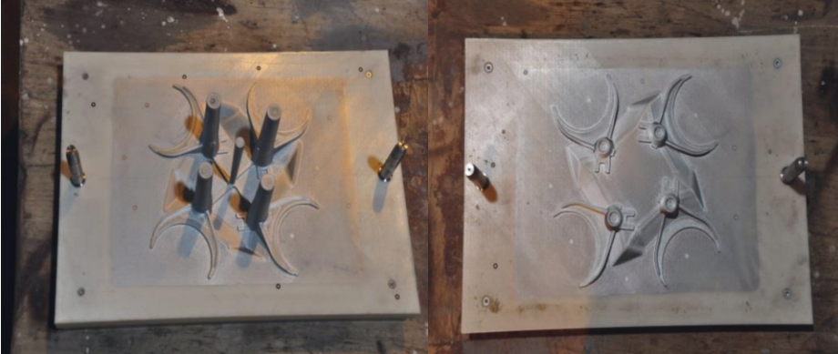
Fig. 3. Derived model for mould making (left: upper part, right: lower part)
