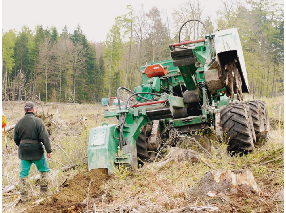
■ Fig. 2.35 Soil milling in strips on a former clear cut in central Germany. (© R. Unseld)
