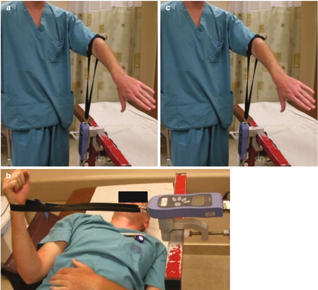
Fig. 2.1 Measurement of the isometric force is performed by a dynamometer with digital record of the generated force over time (sampling 1200/s, 0.04 Newton resolution). For the supraspinatus evaluation (a): the arm is positioned at a 45° abduction and 30° forward flexion in a standing position. The cuff of the measuring device is positioned on the arm. The distance from the middle of the cuff up to 3 cm distal to the acromion (approximate point of the fulcrum of the head of the humerus) is considered as the lever arm length. To measure the strength of the infraspinatus (b) and the subscapularis (c) muscles, the test subject is on his/her back with the tested arm placed
