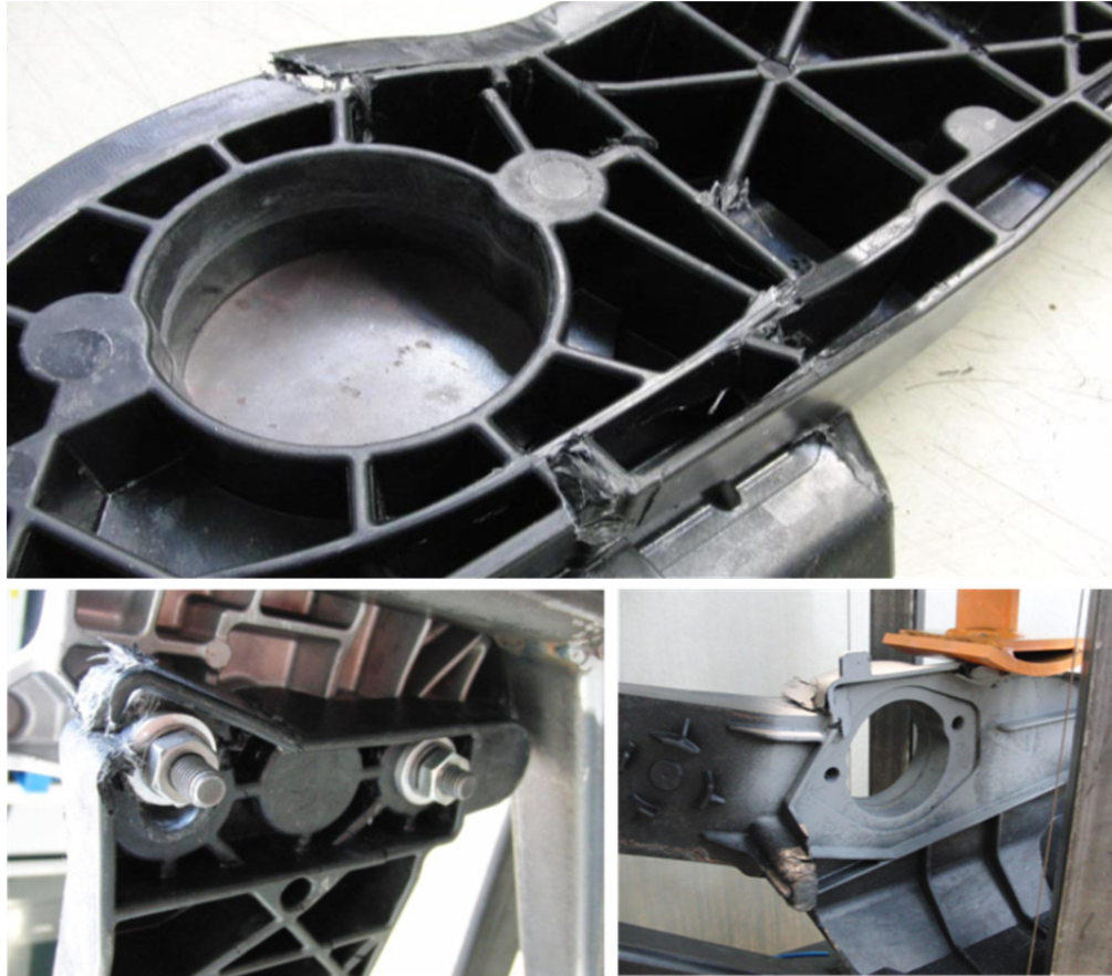
Figure 5: Failure behavior of engine carrier made of gfrp after an impact test
