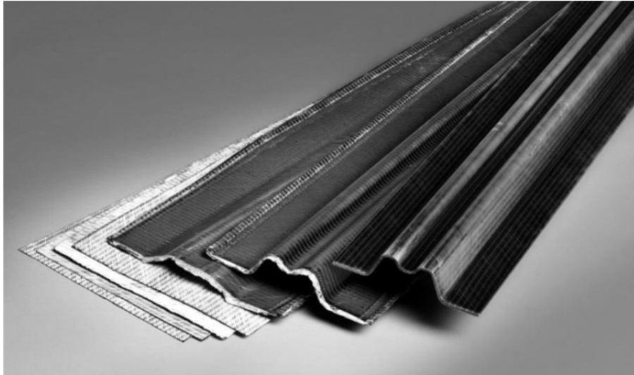
Figure 1: TvD process steps: Prepregs without tack (left), thermoplastically processed semfinished part (mid) and thermoset structural part (right) (last two steps preferably carried out in one step).
