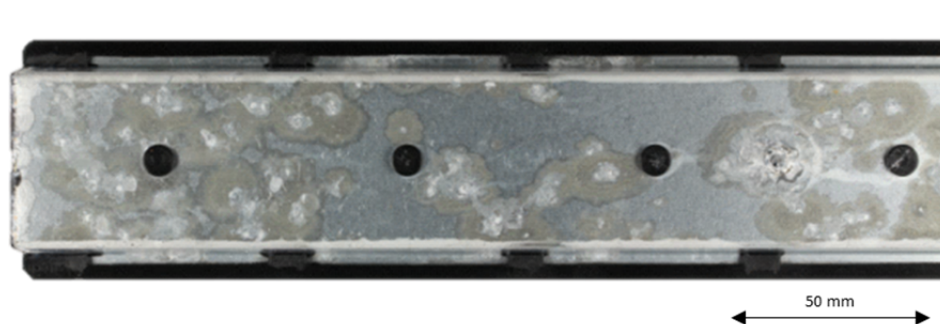
Figure 9: Technology carrier with flatbed lamination after 15 cycles of PV 1210
