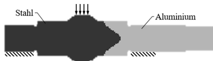
Figure 7: Design result for the demonstrator shaft using IZEO with Tailored Forming restrictions
