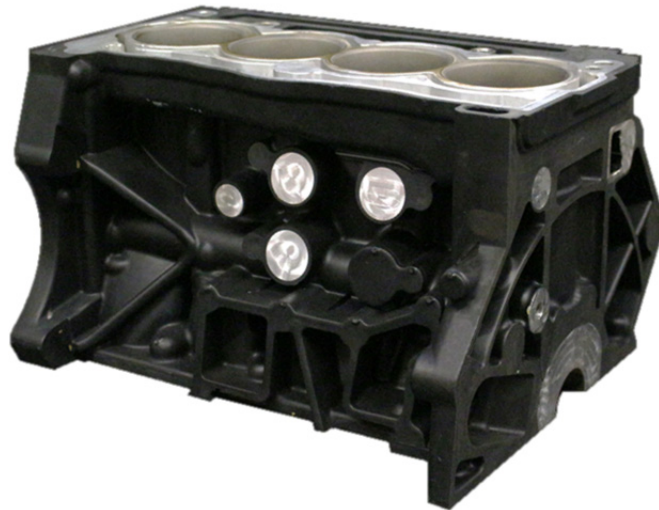
Figure 16: Hybrid cylinder crankcase, pre-manufactured and APS-coated [Volkswagen AG Salzgitter]
