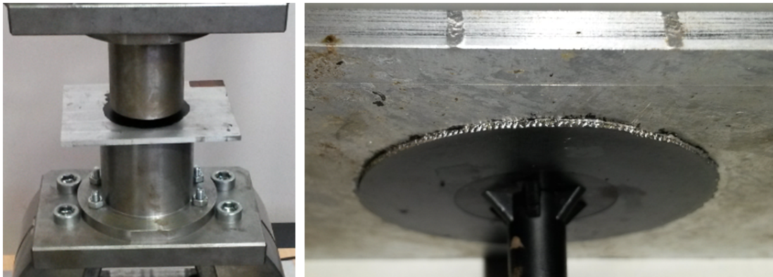
Figure 11: Pressure test (left) and pressed out plastic (right) [Volkswagen AG, Group Research]
