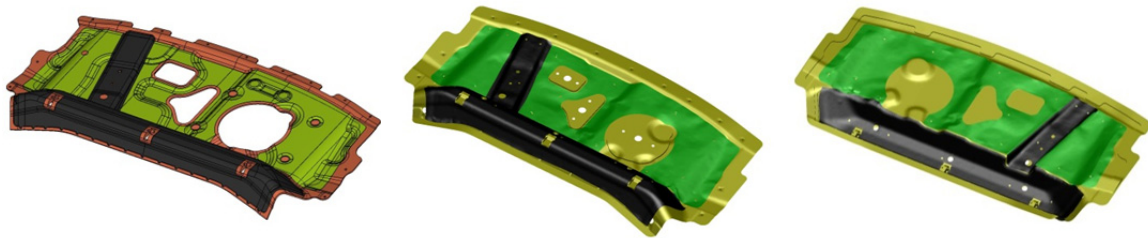
Figure 8: Rear shelf after design (left) with organosheet in black, recycled mat with MuCell process in green and injection molded polymer in brown. On the right side the upper and lower views after performing simulation are shown
