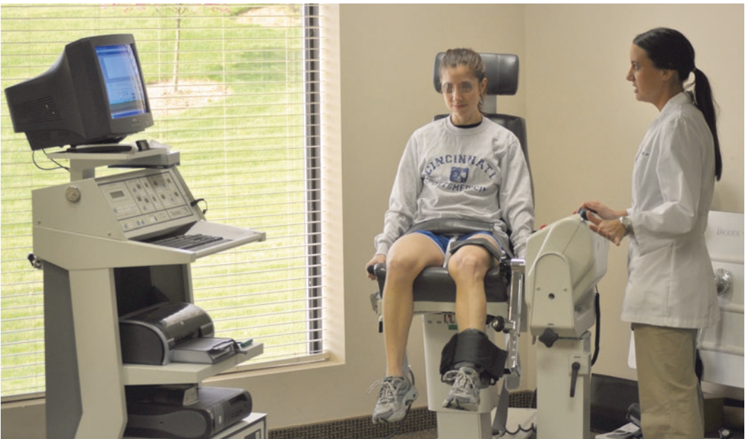
Fig. 21.3 Isokinetic knee flexion-extension strength test on Biodex isokinetic dynamometer (Biodex Corporation, Shirley, NY)
