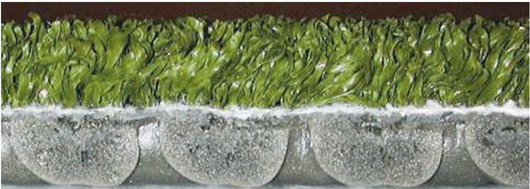
Fig. 5.6 First-generation artificial turf. 10–12 mm fiber length, integral shock pad, nylon, unfilled, hard, and abrasive. Developed in the 1960s [13] (Reprinted by permission of Loughborough University)
