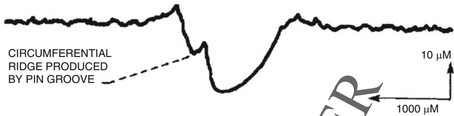
Fig. 3.9 Shows a surface profile of the Sliding contact areas illustrating the wear caused by an embedded hard particle in the UHMWPE disk [29]
