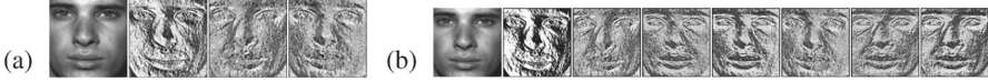
Fig. 4. (a) Sample image and its corresponding LBP and LZZBP images. The 2nd image is the 3 \times 3 LBP image and rest 3rd–4th are 3 \times 3 LZZBP images. (b) The 2nd image is the 5 \times 5 LBP image and rest 3rd–8th are 5 \times 5 LZZBP images.
