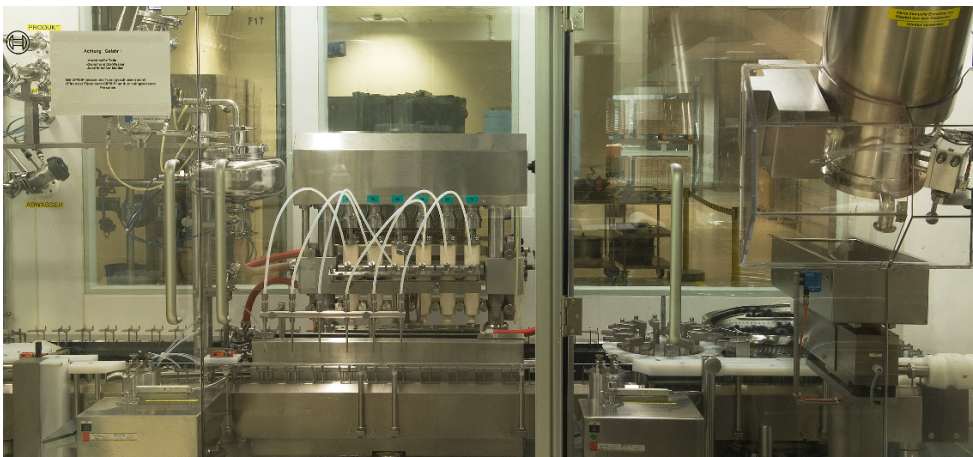
Fig. 14c. Infusion bottle line - filling machine under laminar flow
