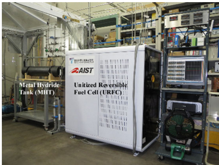
Fig. 13.2 Photo of the THEUS installed in AIST: left, metal hydride tank (MHT); center, unitized reversible fuel cell (URFC); and right, personal computer (PC) for controlling and monitoring the operating parameters
