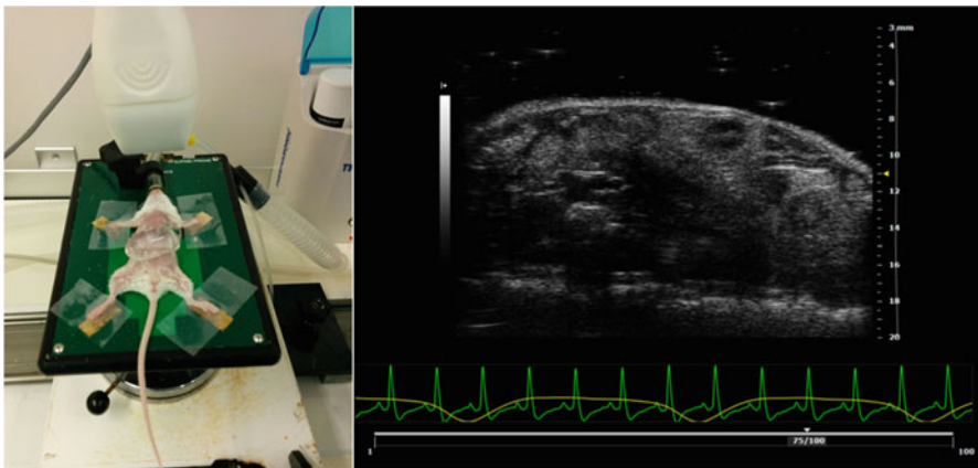
Fig. 8.7 (Left) Mouse positioning and imaging setup (VisualSonics, CA). The limbs are positioned atop electrodes, providing online ECG display. The surface is heated to a user-defined temperature, and anesthesia is applied via a facial mask. The mouse-imaged area is shaved and depilated, and a coupling gel is applied. (Right) A B-mode (reflected waves) ultrasound image of the mouse abdomen scanned using Vevo 2100 high-frequency ultrasound scanner (VisualSonics, CA)
