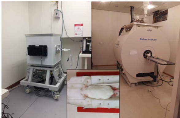
Fig. 8.4 (Top left) Preclinical 1 T MRI system (Aspect, Israel), composed of a permanent magnet. (Top right) Preclinical 9.4 T MRI system (Bruker, Germany). (Bottom) Bruker MRI compatible mouse positioning bed. Anesthesia is provided using a chamber into which the mouse head is inserted. The bed is heated to a user-defined temperature, and respiration can be monitored by placing a sensor close to the mouse chest
