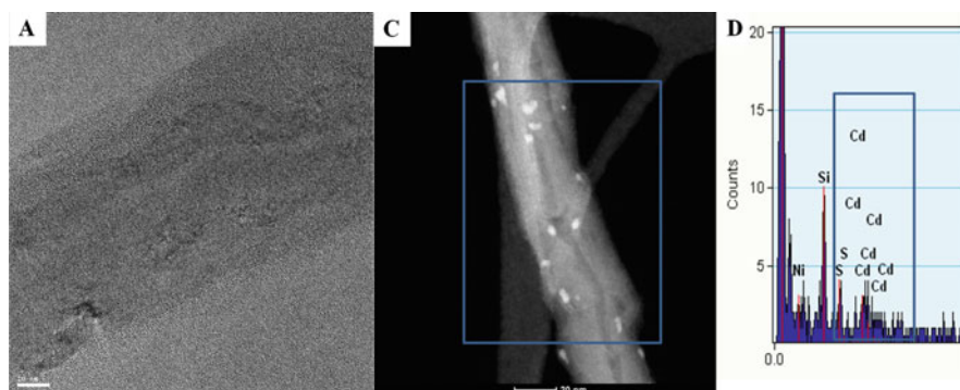
Fig. 8.9 TEM (a) and S-TEM (b) characterization of MWCNTs with CdS-QDs, with the corresponding EDS chemical mapping, showing the presence of Cd
