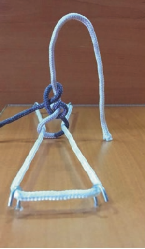
Fig. 6.24 Square knot turns into a sliding half-hitch knot if more tension is applied to one end (in this case, white end).
