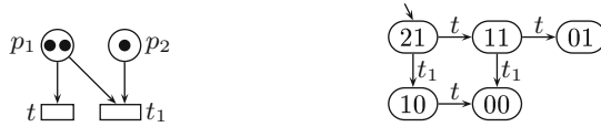
Fig. 4. An example where \{t\} satisfies D0 , D1 , and D2 , but not C1 .
