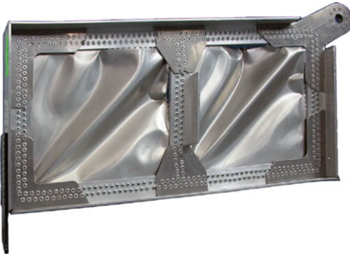
Fig. 9 Complete failure of a shear web assembly; compare (Rammerstorfer and Daxner 2009)
