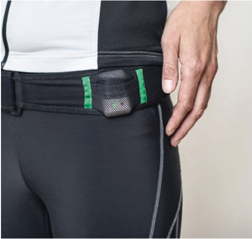
Fig. 8.5 Jump sensor placed in the belt at the position around the subjects' hip
