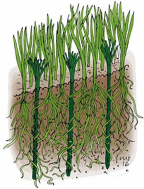
Fig. 30.9 Example of a hybrid playing surface. Sand-based root-zone with long artificial fibres (dark green) to reinforce the natural grass surface (Figure credit Mr. Mike Todd (Brisbane, Australia))
