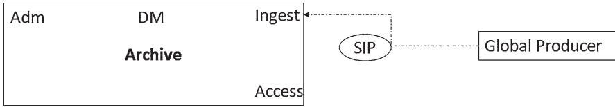
Fig. 15.1 The Submission Information Package (SIP) is sent from the data producer to the archive
