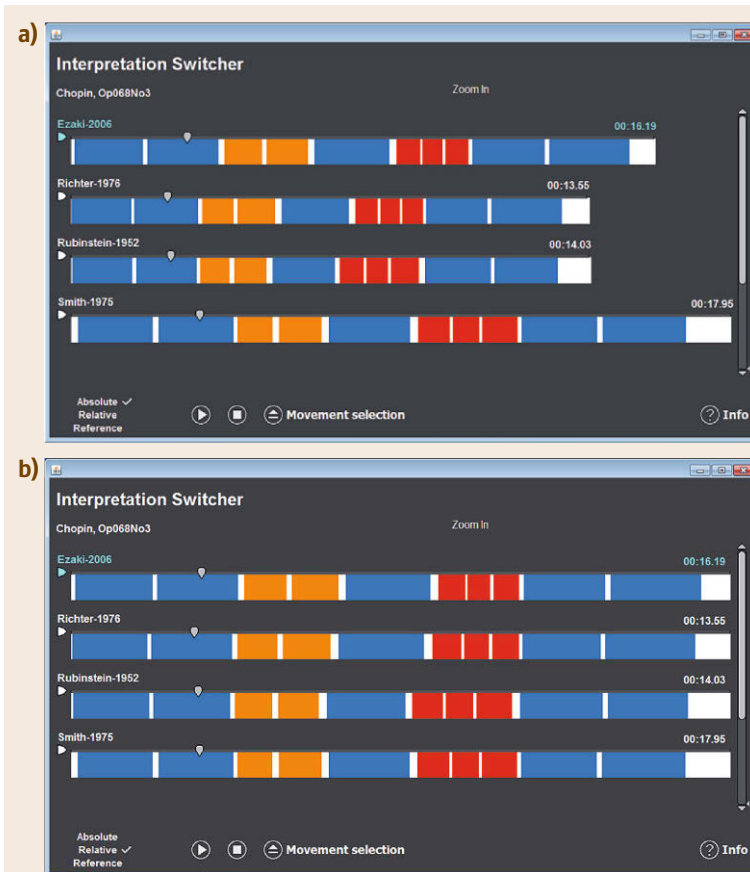
Fig. 39.6a,b User interface for intra- and interdocument navigation of music collections. The slider bars correspond to four different performances of M68-3. They are segmented and color-coded according to the structural annotations in Fig. 39.2. The down arrows point to the current playback time, synchronized across performances. The absolute (a) and relative (b) timeline modes are shown
