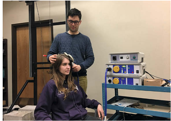
Fig. 27.8 Example of a transcranial magnetic stimulation (TMS) experiment. The experimenter uses a TMS coil to stimulate the participant's premotor cortex (PMC). TMS is a non-invasive stimulation technique used to excite neurons in the cortex by creating a rapidly changing magnetic field at the surface of the scalp
