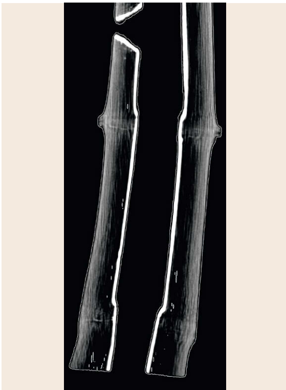
Fig. 4.8 A picture of a computed tomography-scanned old famous ground-paste-free shakuhachi (made by Shinryu Matano (1886–1936) and inscribed as Rodohdoh , 585 mm long, diameter 12–15 mm, in C4). Only the root side is shown. Note that the diaphragms remain a little. The bright layer indicates the urushi coating (courtesy of Hamamatsu Museum of Musical Instruments)
