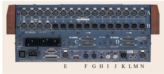
Fig. 12.28 Rear side of a digital mixing console and its typical connectivity (© Yamaha, for descriptions see Table 12.15)
