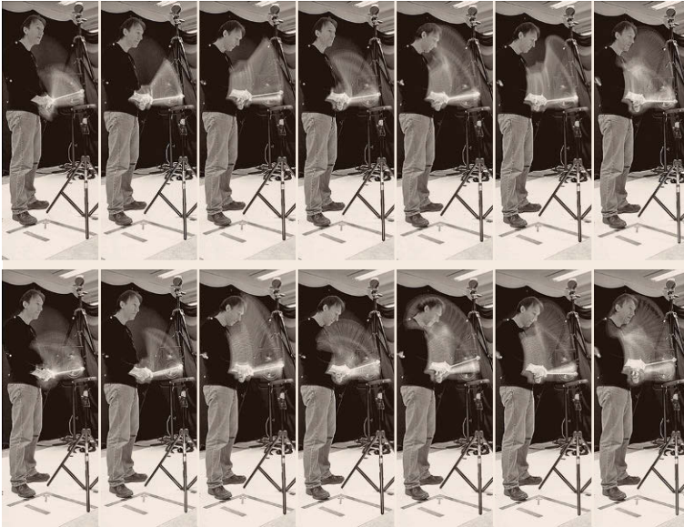
Fig. 38.3 A motion image is created by subtracting subsequent frames in a video file (Frame (2) minus Frame (1))
