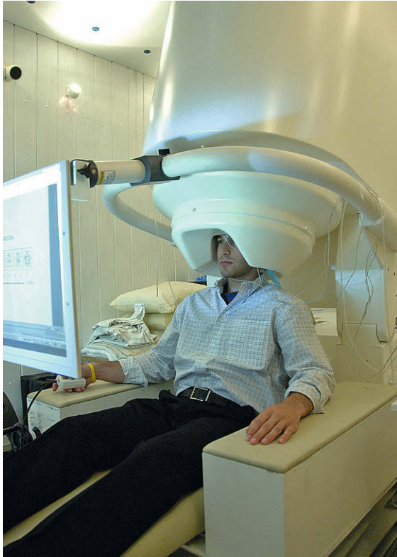
Fig. 27.4 A magnetoencephalography (MEG) machine. Participants sit comfortably in the chair while the large array of sensors, housed in the large white cylinder on the top of the machine, are lowered onto their head. The sensors detect very small changes in magnetic fields caused by neural firing (Photo: National Institute of Mental Health, National Institutes of Health, Department of Health and Human Service)
