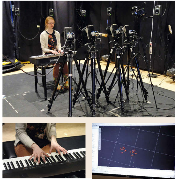
Fig. 38.8 Setup for motion capture of pianist Christina Kobb. In addition to the cameras placed in front, there are also cameras placed behind the pianist to capture the motion in three dimensions
