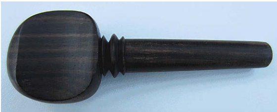
Fig. 4.7 Violin peg turned out of ebony. Ebony can be machined with a sharp edge, as can be seen in the detailing
