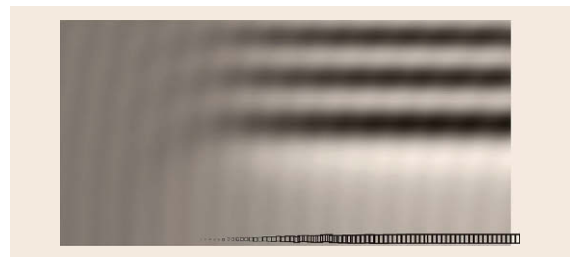
Fig. 18.18 A tapering window eliminates the truncation error but reduces the extent of the listening region (after [18.40])
