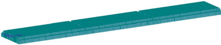
Fig. 10.43 FE model of CRTSII track with three slabs
