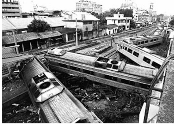
Fig. 1.25 Derailed “Tze-chiang” train on bridge after collided by a truck (news.sina 2011)
