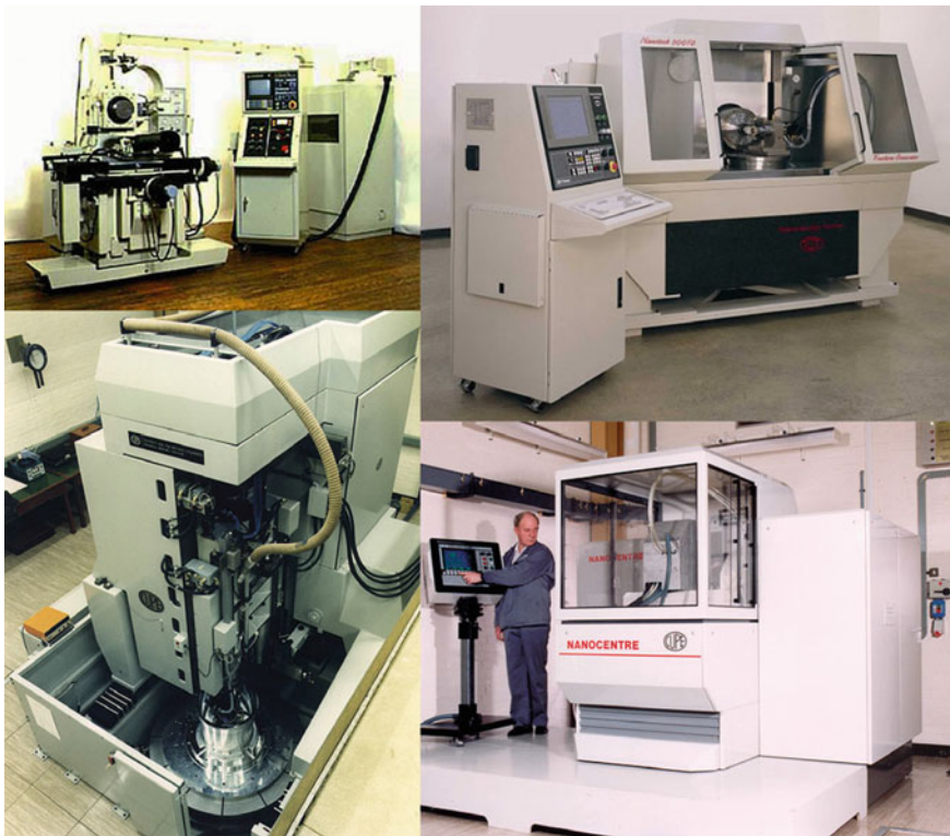
Fig. 1.3 From top left anticlockwise: ca 1975 Moore M18 DTM, Cranfield LDTM (1979), Cranfield NION DTM (1989) and Moore 500FG (1999). Courtesy of Moore, CUPE, CPE Ltd and Moore Nanotechnology Systems (reprinted from the work by Shore and Morantz 2012)
