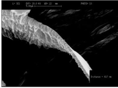
(a) (001) cutting plane; Depth of cut = 5 \mu\text{m}
