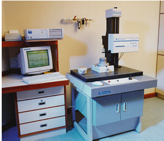
Fig. 4.8 Form Talysurf laser interferometric surface texture measuring system
