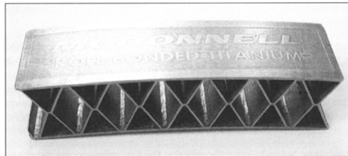
Fig. 3.20 McDonnell Aircraft Astronautics roll-bonded titanium structure (circa 1963), from Advanced Engine Development at Pratt & Whitney SAE Publisher (Mulready 2001). Today, this structure would be superplastically formed and diffusion-bonded from RSR (roll speed ratio) titanium sheets
