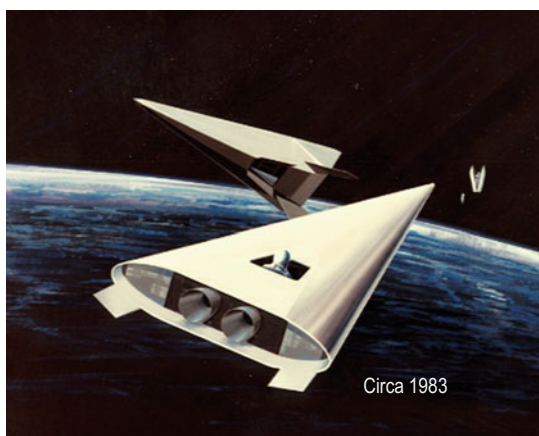
Fig. 2.27 “Bud” Redding’s Space Cruiser launched from a transatmospheric vehicle to accomplish a satellite repair. The Space Cruiser is also able to serve as a three-person rescue vehicle
