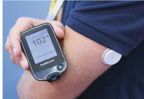
■ Fig. 5.4 FreeStyle Libre (Abbott Laboratories, Wiesbaden). The glucose sensor requires the insertion of a sensor filament under the skin. It can be left in situ for up to 14 days. An additional check of glucose values with a blood glucose meter is required when glucose levels change quickly as the levels in tissue fluid may not represent the true blood glucose levels. The same applies in situations when the system indicates hypoglycemia or a developing hypoglycemia or when symptoms do not correspond with the measured values of the system.
