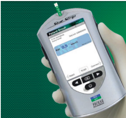
■ Fig. 19.3 StatStrip Glucose/Ketone POCT devices to measure blood glucose and ketones. (With kind permission from Nova, Mörfelden-Walldorf, Germany)
