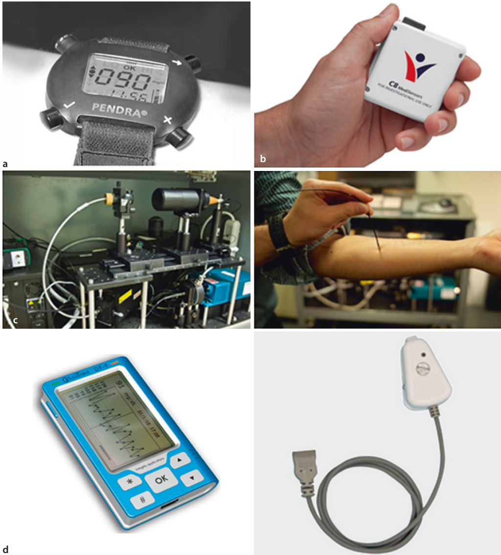
Fig. 11.1a–d Non-invasive analysis methods for POCT devices. a Pendra NGM device. b HG1-c, Continuous NGM device, manufactured by C8 MediSensors. c Prototype of a Raman spectroscopy-based NGM sys-
