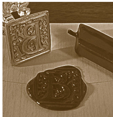
Fig. 5.1 Printing a seal into viscous wax is a way of replication using hot embossing. The figure shows a seal (stamp), wax tube (candle), and embossed pattern
