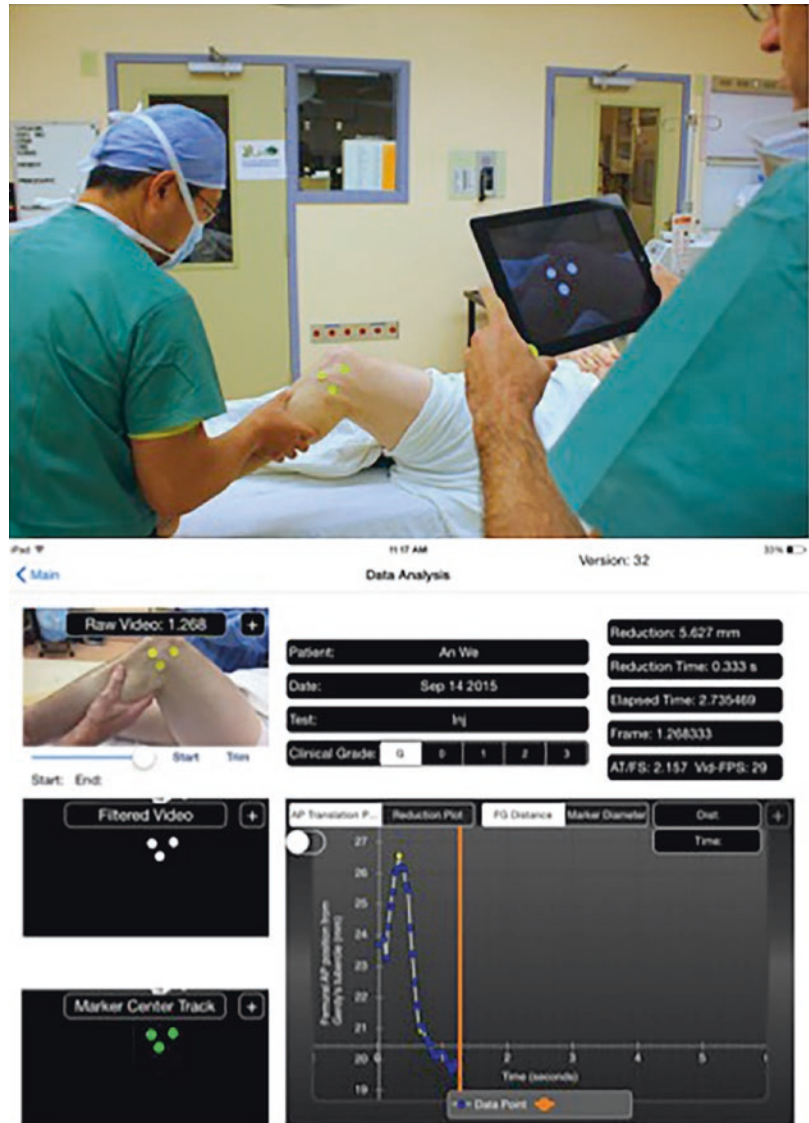
Fig. 51.6 Intraoperative pivot-shift measurements with electromagnetic motion trackers and quantification with iPad software
