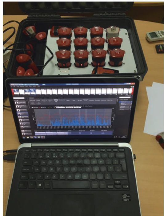
Fig. 32.4 GPS monitoring system with player's training raw data
