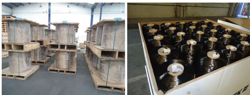
Fig. 9.5 Softwood kraft lignin: PAN (25:75) based precursor ( left ) and carbonized fiber ( right ) produced in commercial spinning and carbonization equipment by Zolcor–Weyerhaeuser collaboration. Reproduced from Husman [248]
