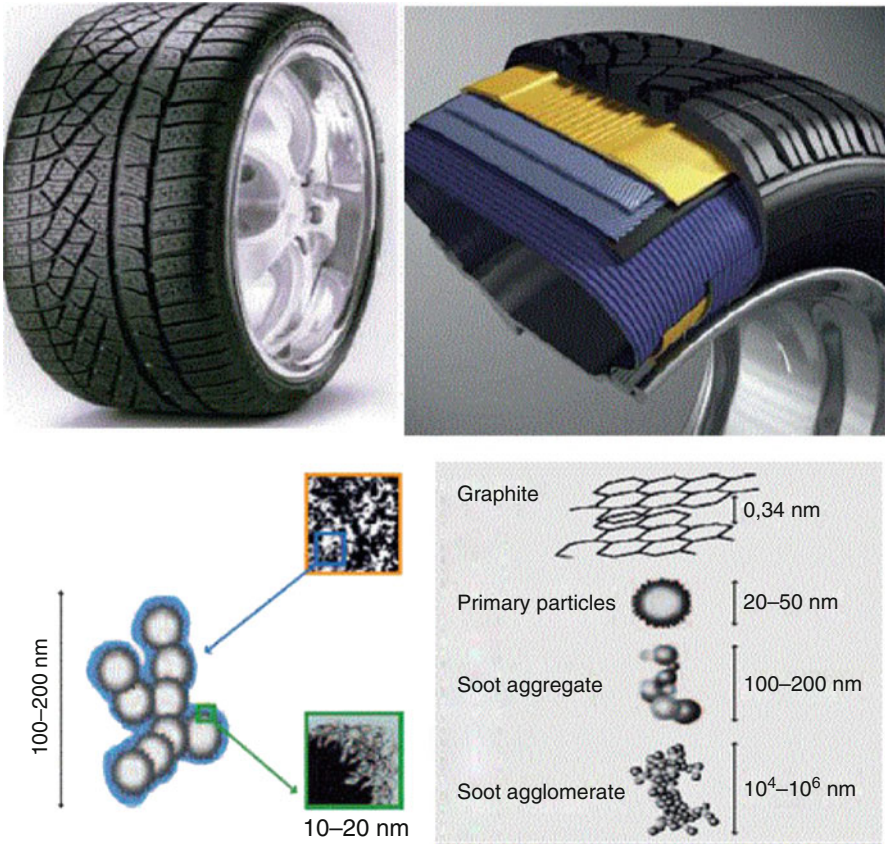
Fig. 7.12 Schematic illustration of a modern nanostructure-based tire for cars [08Das, 10Zho]
