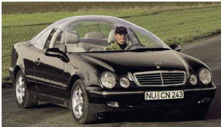
Fig. 7.18 Modern automobiles equipped with nanostructured polymeric glasses for roof, windows, and cover light
