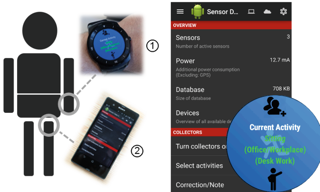
Fig. 5. Collector and labeling framework: Wear App (smart-watch, 1) and Hand App (smart-phone, 2). Our app is online available. ( https://play.google.com/store/apps/details?id=de.unima.ar.collector&hl=en )
