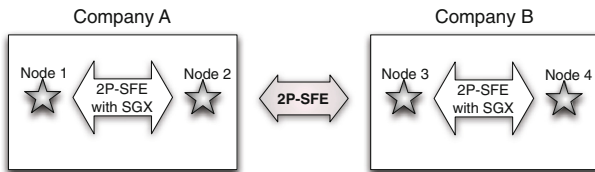
Fig. 1. Half and Half. In this usage, we convert SGX-supported 2P-SFE values to standard 2P-SFE values and back in order to take advantage of the speed of the combined form when the trust model is acceptable and still allow for a stronger model when the trust model of SGX-supported 2P-SFE is not acceptable (say, the user does not trust Intel when using a public network).
