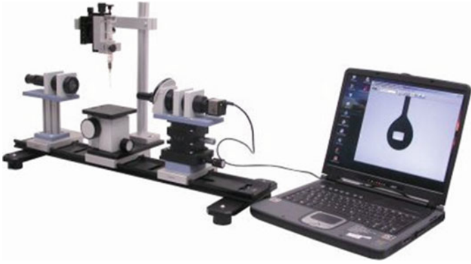
Fig. 4.11 A video system used for drop shape measurement
