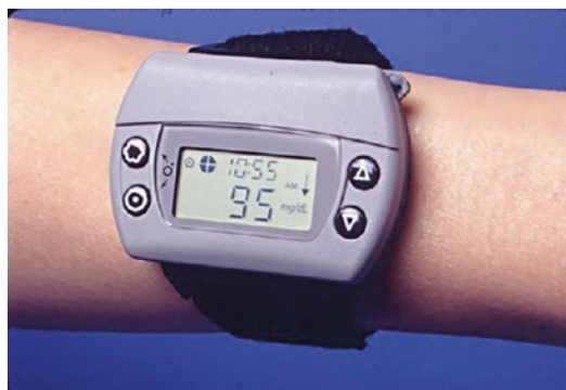
Fig. 6.7 The GlucoWatch G2 Biographer developed by Cygnus, Inc. (USA), and approved by the FDA in 2001 was a glucose monitoring device which allowed non-invasive glucose monitoring through the skin (Image kindly provided by and with permission from Dr. R. Potts)
