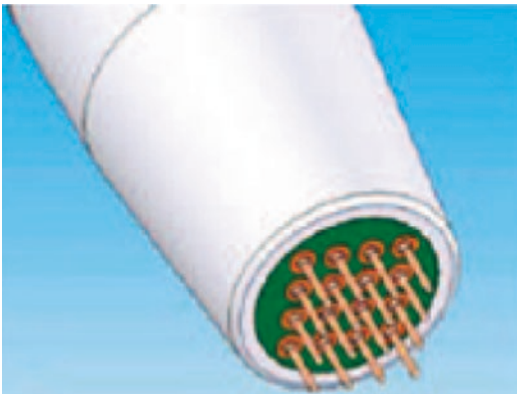
Fig. 8.7 A prototype development of minimally invasive 4×4 array trocar-gold-coated electrodes for intradermal applications (Invio® Pharmaceuticals, USA) (Reproduced from Broderick et al. 2011, 261. With kind permission from Nature America Inc., USA)
