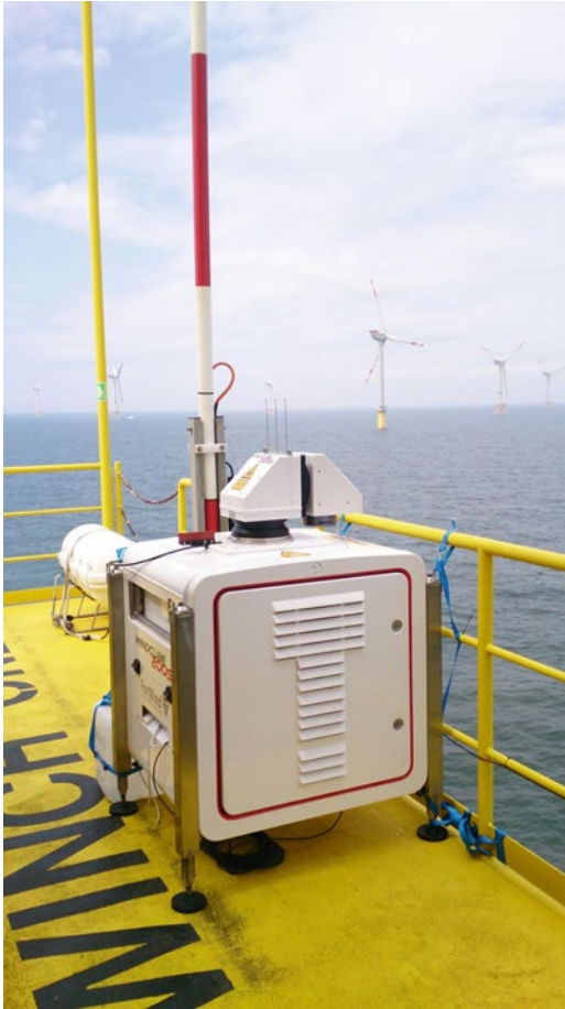
Fig. 13.1 Long-range lidar on the Alpha Ventus transformer platform. © ForWind – University of Oldenburg
