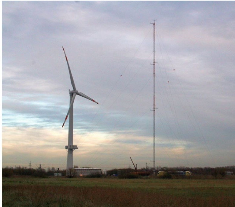
■ Fig. 12.4 First measured prototype in Bremerhaven and the met mast. The lidar (not visible in the photo) is located about 10 m from the met mast. © SWE University of Stuttgart
