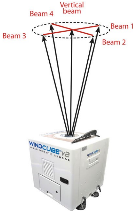
■ Fig. 12.1 Measurement principle of the lidar system. © Leosphere
