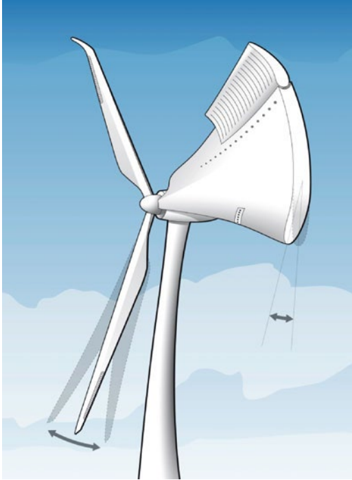
Fig. 10.2 Active rotor blades adapt to the wind strength. © DLR; Lizenz CC-BY 3.0
