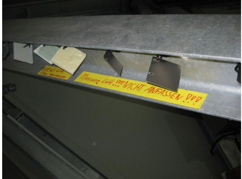
■ Fig. 26.1 Attachment of the material samples on a supporting beam in the nacelle of AV7. © fk-wind:
