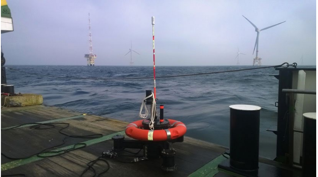
■ Fig. 13.3 The measuring buoy used in the GW Wakes project before it was positioned near the Fino 1 research platform. © BSH
