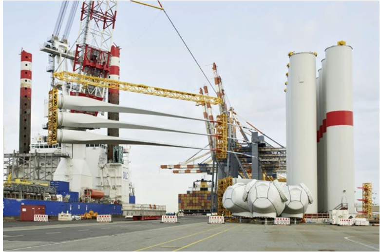
■ Fig. 9.1 Rotor blades being loaded for installation in an offshore wind farm. © Senvion GmbH 2015
