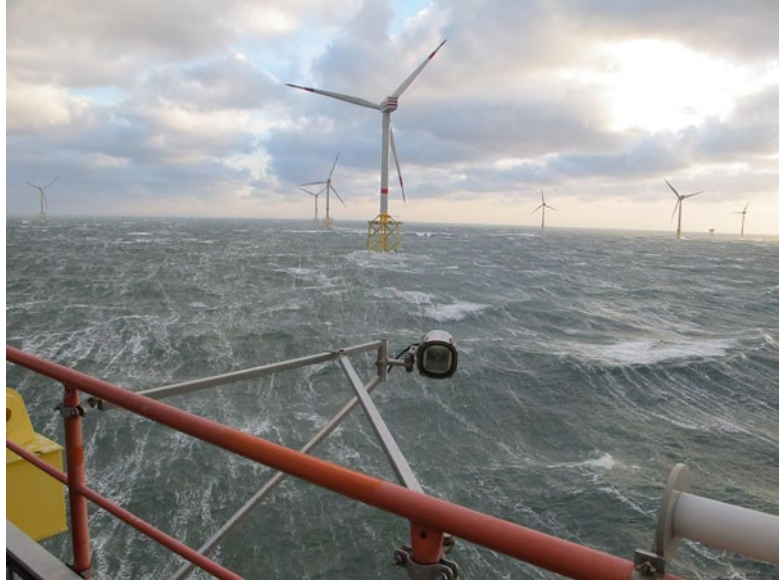
■ Fig. 21.5 Camera on the Fino 1 research platform for observing sea birds. © Marine Monitoring Networks/BSH
