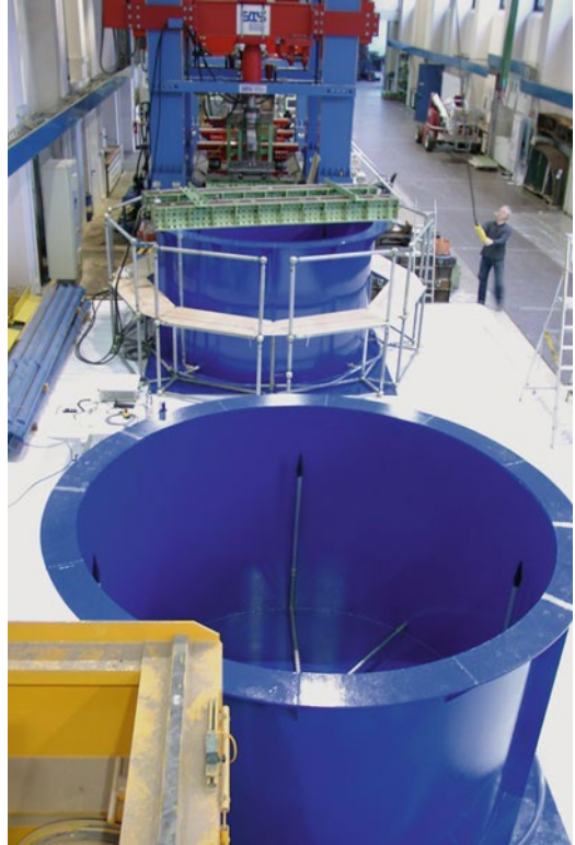
▣ Fig. 6.5 Preparation of trial boxes for testing laterally loaded piles. © BAM
