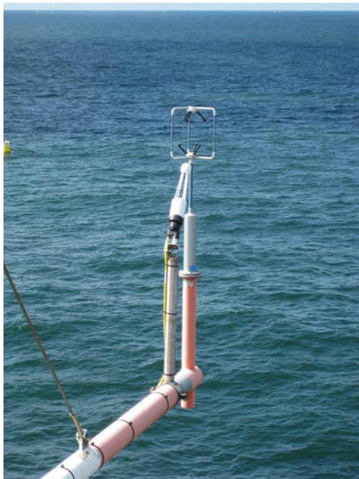
■ Fig. 17.1 Measuring arrangement for high-resolution moisture measurement on Fino 1 at a height of 41.5 m. The humidity was measured with the white device in the foreground using optical absorption, and behind it is an ultrasonic anemometer for measuring wind speed fluctuations. © UL International GmbH (DEWI)
