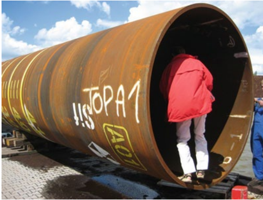
▣ Fig. 6.4 Checking the instrumentation on a tripod pile. © BAM
