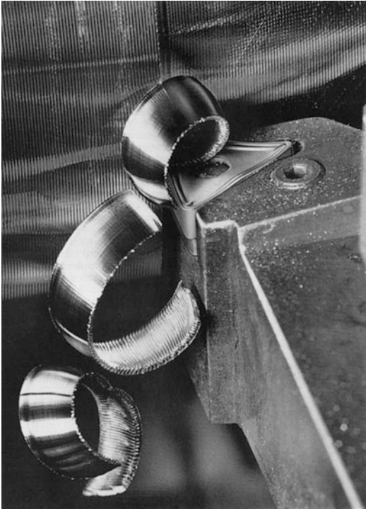
Chip-Forms, Chip Breakability, and Chip Control, Fig. 8 3D chip breaking from optimally designed cutting edge configuration and chip groove (Sandvik 1996)
