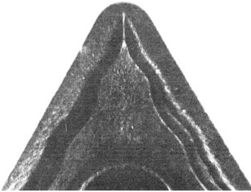
Chip-Forms, Chip Breakability, and Chip Control, Fig. 5 Complex chip-groove geometry in a cutting tool insert
