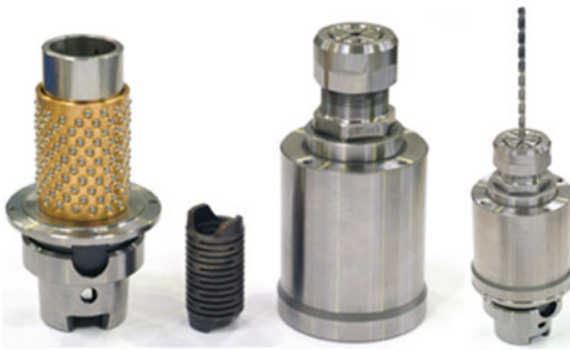
Self-Vibratory Drilling, Fig. 6 Components of SVDH and SVDH with a twist drill
