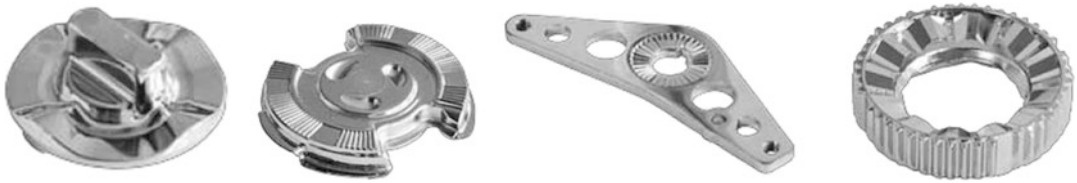
Sheet-Bulk Metal Forming, Fig. 1 Examples of sheet-bulk metal forming parts with functional elements (Feintool 2015)
