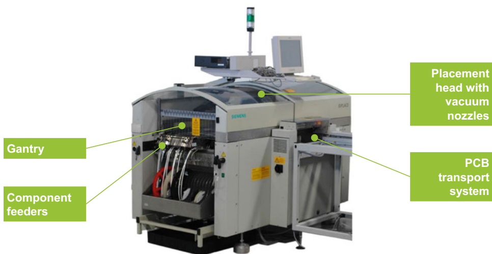
SMD Component Placement, Fig. 1 Functional elements of SMD placement machines
