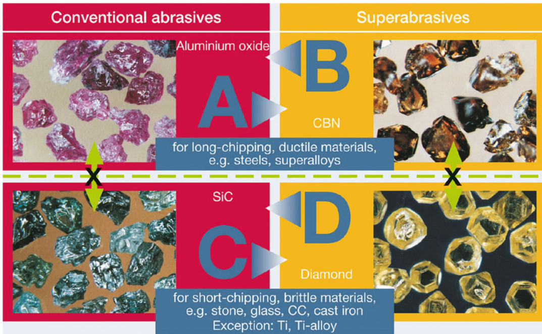
Superabrasives, Fig. 5 Classification of abrasive grains with standardized letter symbols and application areas, (Helletsberger et al. 2011) (With copyright permission from publisher)
