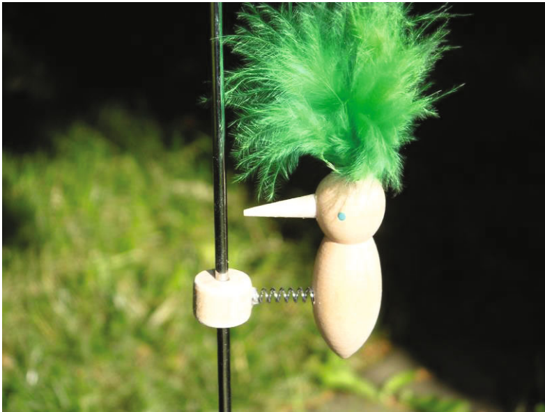
Fig. 12.10 At rest, this system is “self-braking.” If one swings the bird, the self-braking is intermittently removed and the fastener slides down the rod. This alternating change between sticking and sliding is an example of a sprag-slip movement.
