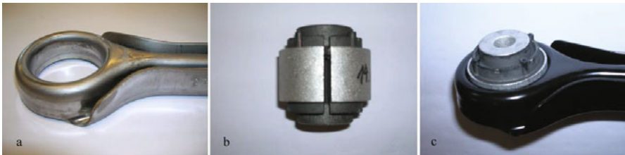
Fig. 10.16 (a) Wishbone with sheet-metal eyelet; (b) Slotted rubber-metal bearing; (c) Finished wishbone with press-fitted bearing.
