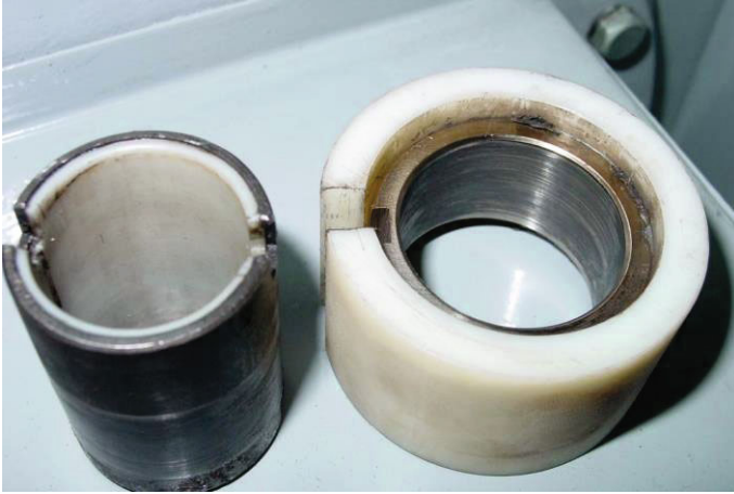
Fig. 12.5 Part of a bush bearing made of manganese steel for which the installation of a correctly dimensioned polymer lining has suppressed squeal.
