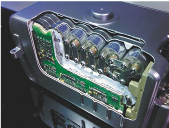
Fig. 8.1 Lithium-ion battery system with a block design, Daimler S400 hybrid (courtesy of Daimler AG)
