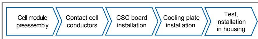
Fig. 17.7 Battery module assembly
