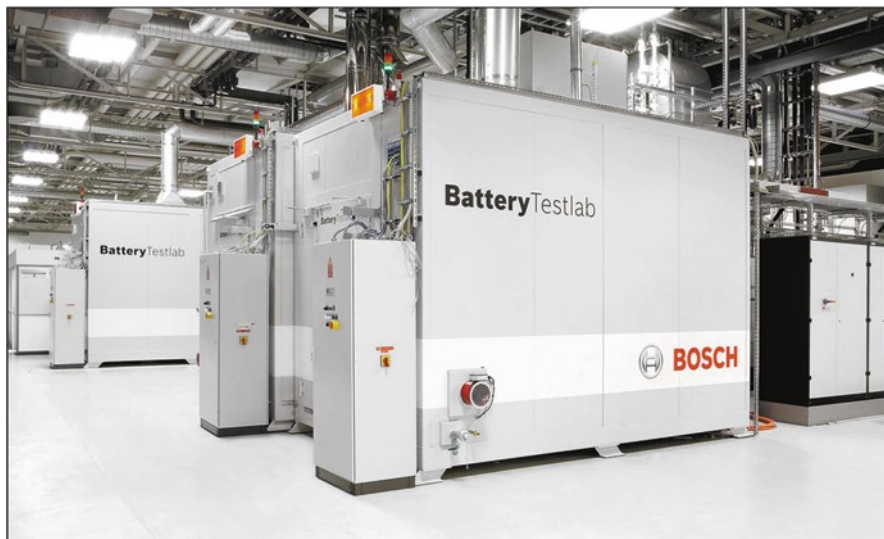
Fig. 25.7 Research laboratory test facilities for cell tests ( Source Bosch)
