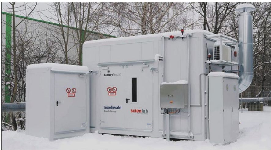
Fig. 25.9 Cell test facility with a disposal storage unit (moehwald/scienlab)
