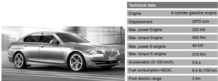
Fig. 31.5 The BMW Active Hybrid 5 and its technical data used for battery development
