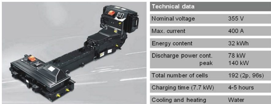
Fig. 31.8 The lithium-ion battery of the BMW Active E and its technical data
