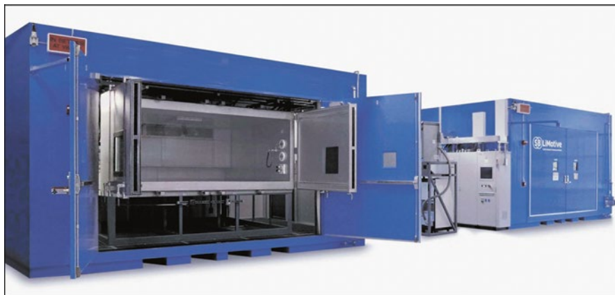
Fig. 25.6 Pack test system for commercial vehicles, stationary plants, and batch tests (Cobasys Research Laboratory, Michigan, US, Source BOSCH)
