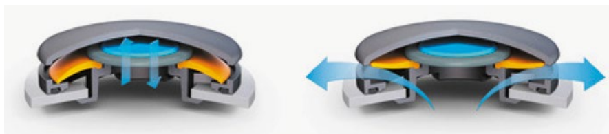
Fig. 10.6 “DIAvent” element for pressure regulation and overpressure release. In normal operation, pressure regulation is performed through an IP 67 proven non-woven section (gas transfer typically 8 liters per minute). In case of overpressure release, an umbrella valve can be activated (activation pressure typically 50 mbar; gas throughput typically 40 liters/sec).
