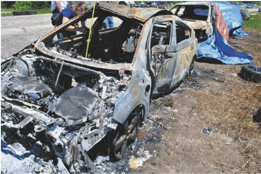
Fig. 21.2 Electric vehicle after a battery fire following a crash test. The subsequent fire spread to four nearby vehicles [1]
