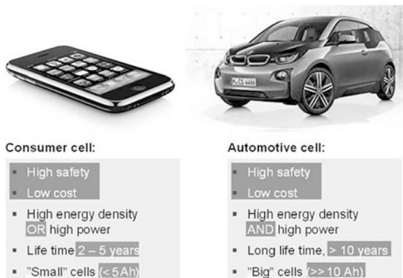
Fig. 31.11 Major differences between using lithium-ion technology in consumer products and in the automotive industry
