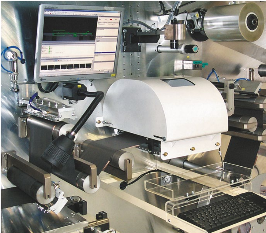
Fig. 19.2 Inline electrode geometry measurement. The anode band being measured is moved from left to right [4]
