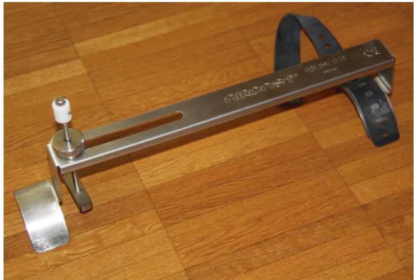
Fig. 38.2 The Rolimeter ® : a simple device to measure anterior knee laxity
