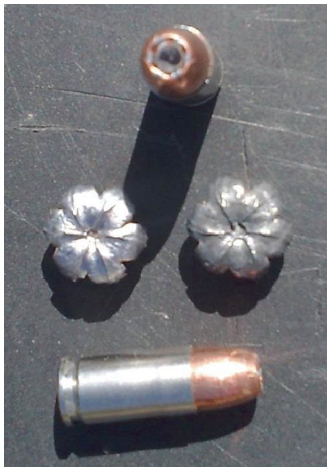
Fig. 24.2 Handgun bullet designed to open on impact and increase its cross-sectional area, often used for self-defence
