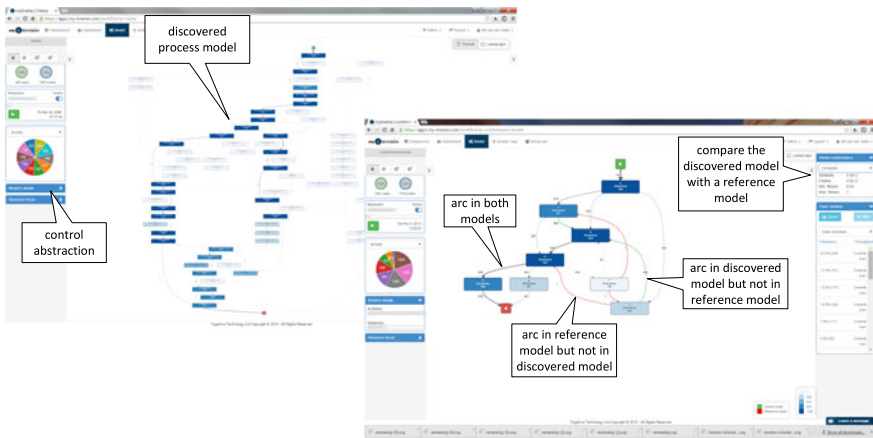
Fig. 11.15 A process model discovered using myInvenio (left) and the comparison of a reference model and a discovered model (right)
