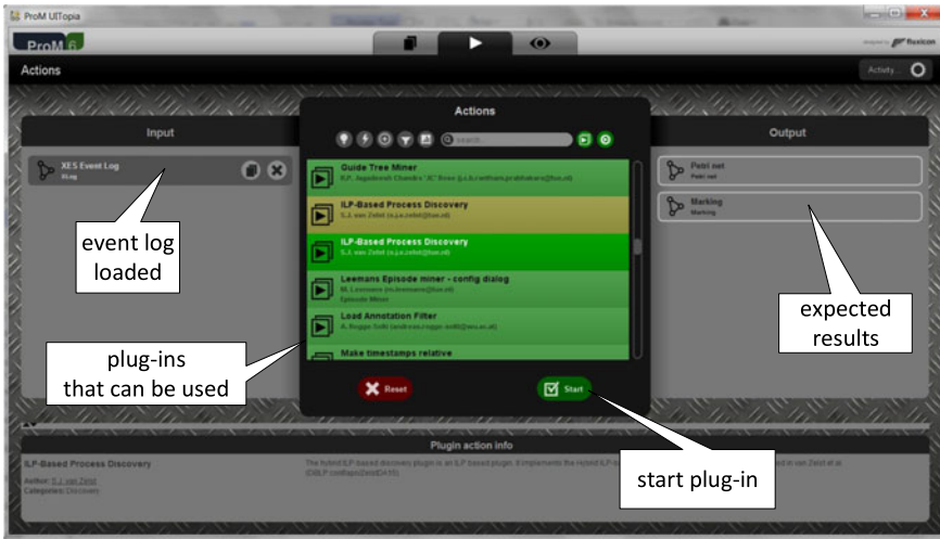
Fig. 11.3 Screenshot of ProM 6.5. After loading an event log, a list of applicable plug-ins is shown and the plug-in implementing discovery using language-based regions (ILP miner) is selected
