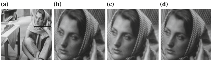
Fig. 5 S = 0.6 , The reconstructed image of Barbara. a Original image of Barbara. b BCS-SPL, PSNR = 30.27 dB, SSIM = 0.90798. c MS-BCS-SPL, PSNR = 30.57 dB, SSIM = 0.89698. d TO-BCS-SPL, PSNR = 30.70 dB, SSIM = 0.9364
