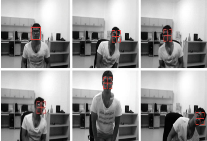
Fig. 2 The improved template matching tracking algorithm
