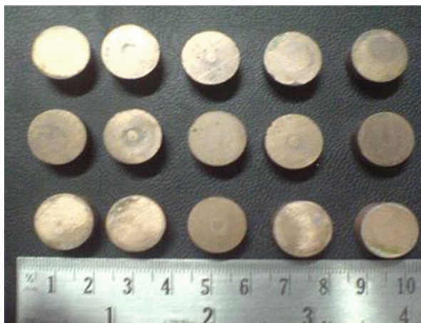
Fig. 13.4 Typical copper–graphite composite processed through P/M route
