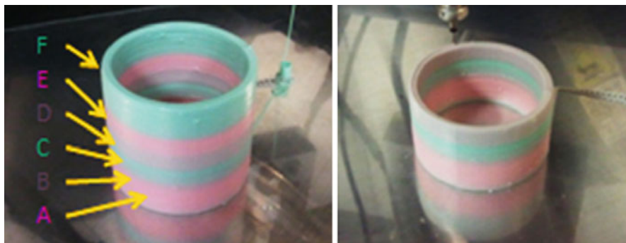
Fig. 4.18 Extrusion of pink- and green-colored \text{CaCO}_3 pastes for tests with and without mixing [98]
