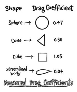
the drag force increases with the velocity squared: the drag coefficient c. Companies put a lot of effort into optimizations of the designs of cars, trains and other vehicles. You can vary your own shape when the next strong wind blows and test the drag coefficients that we provided.
