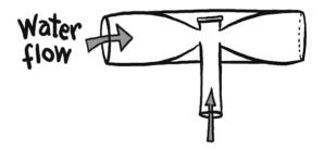
does a plane fly?" ( $\checkmark$ 2). Another nice application is the Venturi tube. The tube has a more narrow part in which the liquid has to flow faster and causes a pressure drop. If you connect a second tube to that part, you can inject a second fluid via the depression, for instance. Such Venturi tubes are used to mix gasoline and air within a combustion engine or to add air to wine to make it taste better.
