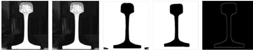
Fig. 44.3 The process of the algorithm, from left to right a input image with light source in the daytime, b median filter c, binary image, d morphological denoising with “X”, e end face contour
