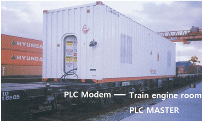
Fig. 76.8 Reefer container monitoring system using PLC-based technology for train
