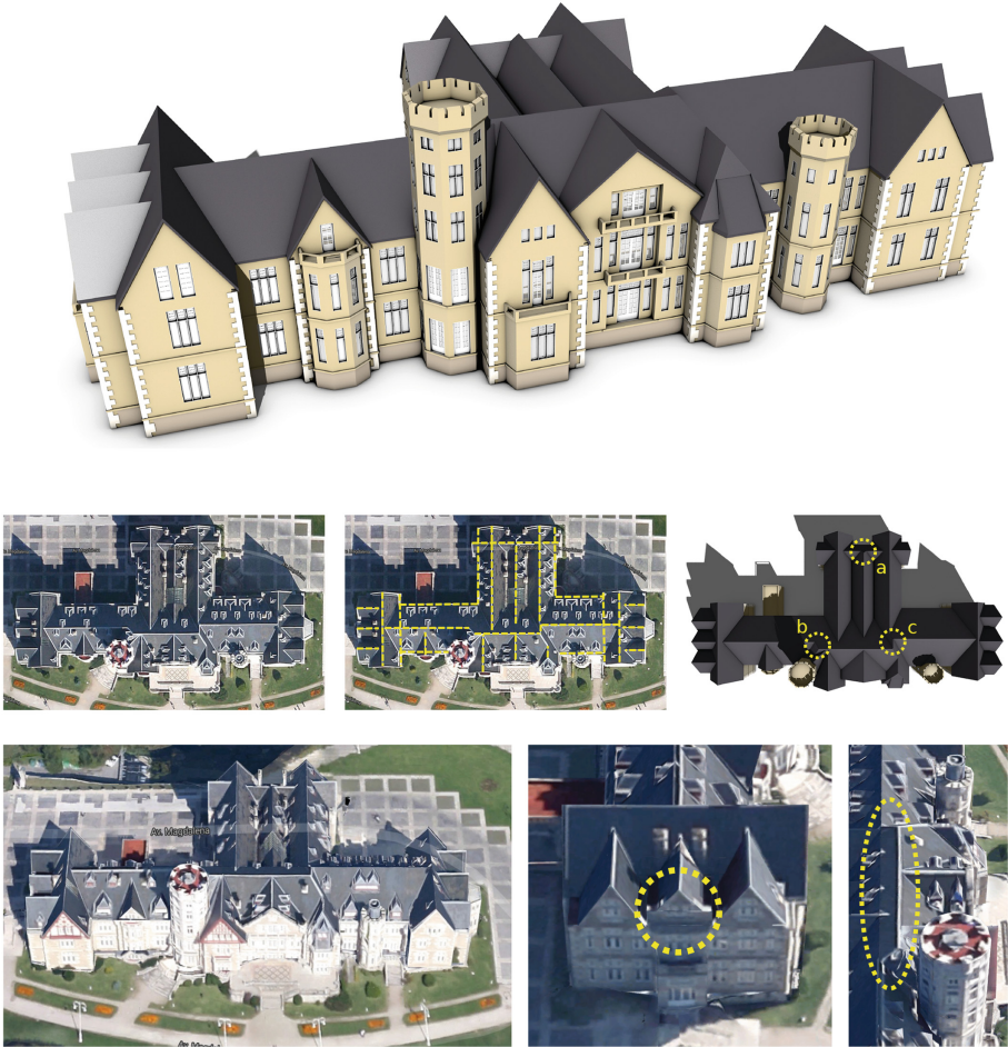
Fig. 21. Model of the Magdalena palacio in Santander, Spain (as in the teaser - Fig. 1). The modeling process was done with aerial images (middle left, middle middle) as in Fig. 19. The detail of the model is increased with existing procedural approaches. Here we used a conventional shape grammar approach for modeling the facades (top). The model has three cases where roof topology changes because of a specified trimming (middle right - marked with yellow circles). (a) is the top row case from Fig. 9, (b) is the middle row case from Fig. 9, and (c) is a complex case where five solids with different trimming specifications are involved. The bottom row shows the 3D model in Google maps on the left. Again the constraints of planarity of roof faces and straightness of edges are not satisfied. Two additional regions with wrong geometry are emphasized in yellow circles. Aerial images: Map data ©2015 Google, basado en BCN IGN España.
