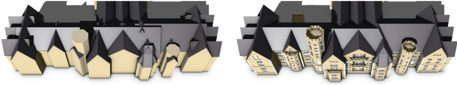
Fig. 1. Modeling a building by parametrizable parts greatly reduces the necessary effort. A simple union of parts might lead to undesirable results (left). Therefore, we introduce automatic roof trimming for solid building primitives. The resulting model can be further refined using existing procedural approaches (right).
