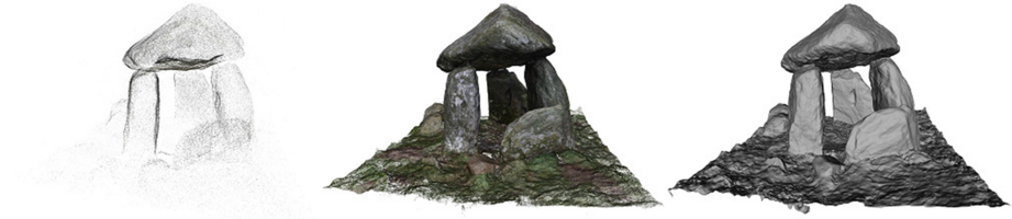
Fig. 4. The sparse point cloud (left), dense point cloud (centre), and untextured mesh (right) generated for Bodowyr Burial Chamber.
