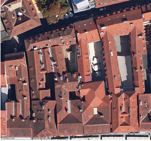
Fig. 4. Aerial image of the inner city of Graz, Austria. Different roof parts merge and form a complex roof landscape. There are many implicit dependencies of parameters of roof faces like slope, height of eave, etc. This roof landscape is not easily created with existing modeling tools. Imagery ©2015 Google, Map data ©2015 Google.
